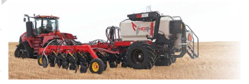
The HD ParaLink<sup>™</sup> hoe drill version of the FMS allows the Operator to seed with all of the benefits of independent seeding. The HD FMS deploys the one-to-one PLX Seed Opener Assembly.
